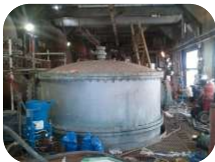
Ammonia distiller operating at 95-100°C had become badly corroded due to the harsh operating environment. The internal surfaces were abrasive blast cleaned and coat using 205 Ceramic HT Fluid
