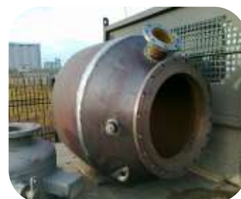
Process vessel operating at 95°C relined using 2 coats of 205 Ceramic HT Fluid
