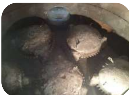
Ammonia distiller operating at 95-100°C had become badly corroded due to the harsh operating environment. The internal surfaces were abrasive blast cleaned and coat using 205 Ceramic HT Fluid
